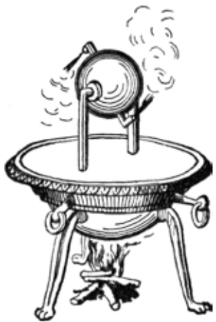
HERO'S AEOLIPILE Knight's American Mechanical Dictionary, 1876.
